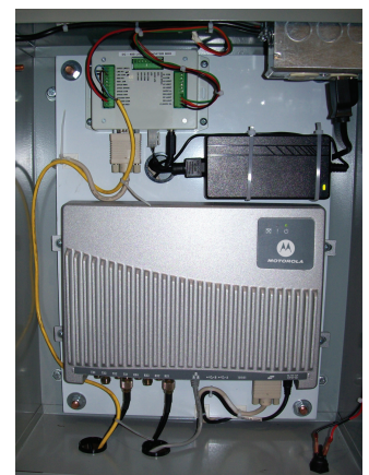
Motorola fixed readers are housed in industrial boxes. A light box above the reader visually indicates RFID tag reads.
